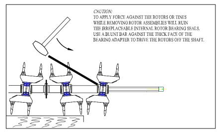
Figure 7. Disassembly of Rotor Shaft Assembly
